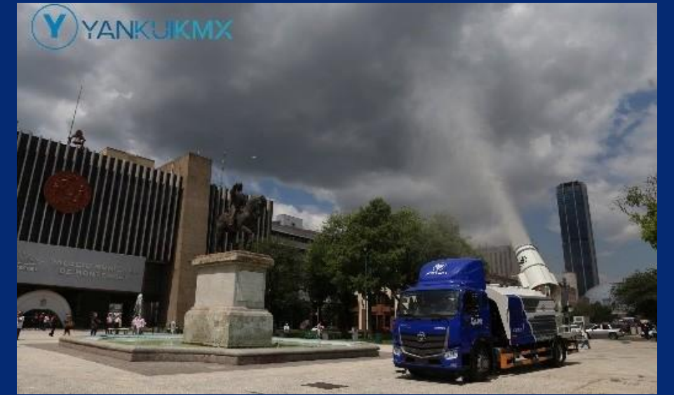
Multifunctional dust suppression vehicle for urban disinfection in Mexico.
